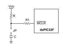
Note 1:  $R \le 10 \ k\Omega$  is recommended. A suggested starting value is  $10 \ k\Omega$ . Ensure that the MCLR pin VIH and VIL specifications are met.
